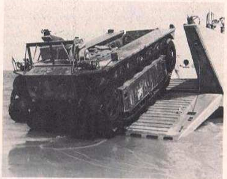
During LOTS testing the MTV disembarks over-the-ramp of an LCM-8.
