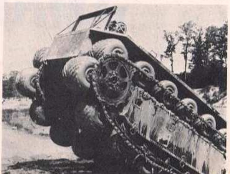
The MTV climbs a steep canal bank after completing swimming trials.
