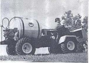
Versatility is PUG's second name. If there's a job to do, just call on the PUG. You can attach a harrow or chisel plow and till fields. Mount your spraying equipment on the rear section and you can move through your shrubs and plants a lot easier and faster. No need to own a special mower because you can attach a large size rotary to your PUG and do the job better.
