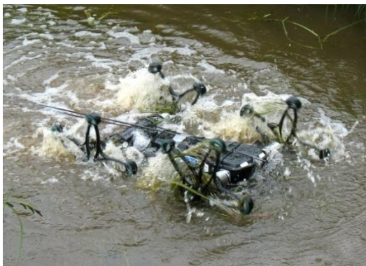
ASGUARD has a waterproof body and is able to swim.
