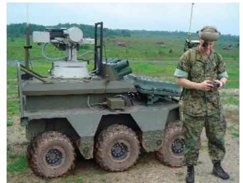
(Above) Gladiator, an unmanned robotic vehicle that exhibits high mobility and advanced robotic scouting capabilities required for the Ground Combat Element of the United States Marine Corps.
