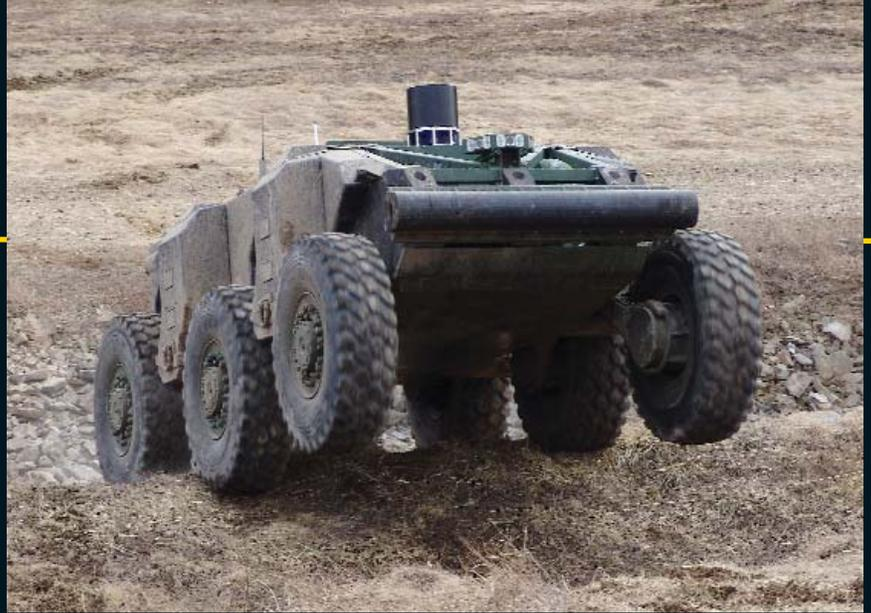
*Crusher's suspension system allows it to maintain high offroad speeds across extreme terrains.*
