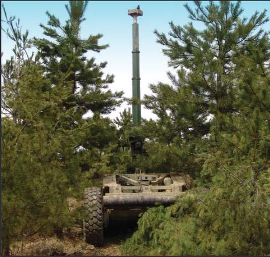
18-foot telescoping mast enables covert surveillance in dense environments.
