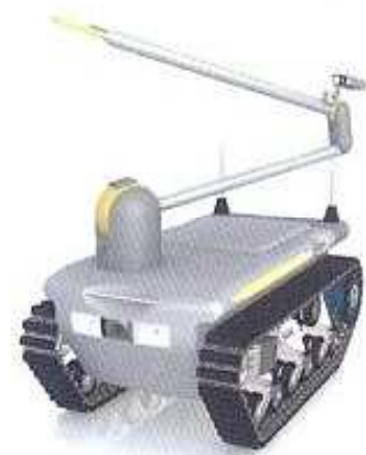
IQbot featuring HAPSITE® integrated chemical sensor
