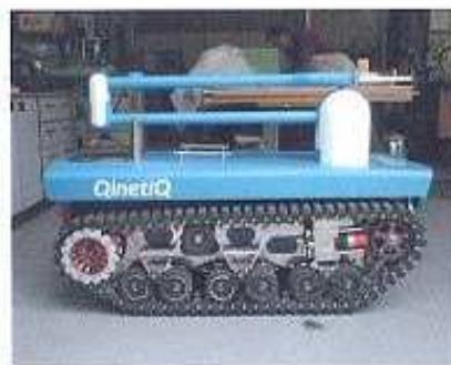
IQbot hermetically sealed hull, standard track and drive modules
