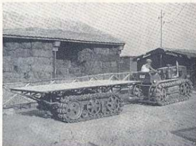
Figs. 7 and 8 (Left)—Lombardini Castoro tractor with the Bonmartini pneumatic track: the track lubricating pump can be seen at the front wheel. (Right)—Fiat 25C tractor and trailer with the Bonmartini roller track
