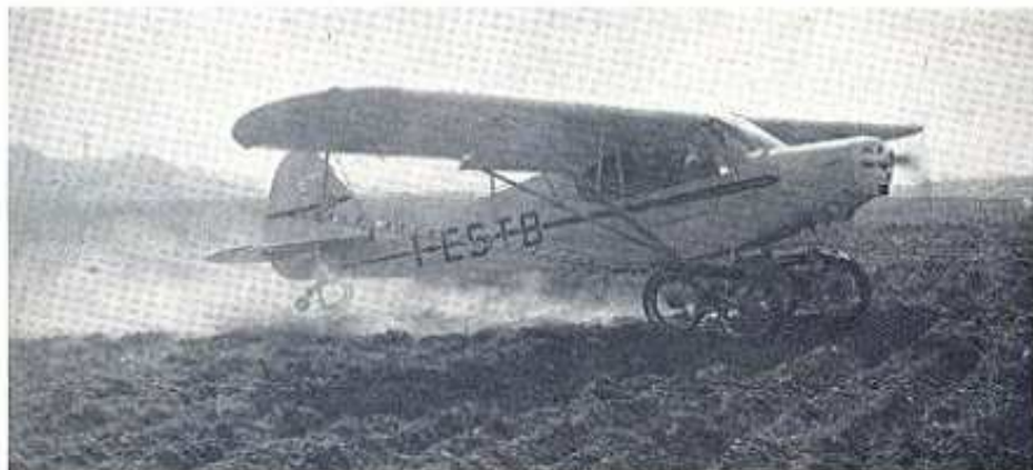
Fig. 5—Piper light aircraft with the Bonmartini track taxiing across a ploughed field
