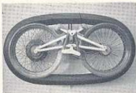
Fig. 6—Aircraft landing gear with the Bonmartini pneumatic track
