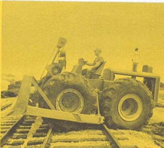
Crosses tracks without damaging ties, tripping signals, tearing rails loose, or injuring tires.
