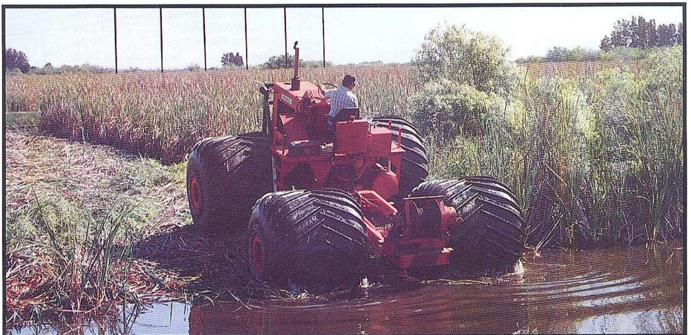
Rolligon standard 4 x 4 Roughneck vehicle with Rolligon 72 x 68 - 28 high flotation tires.
