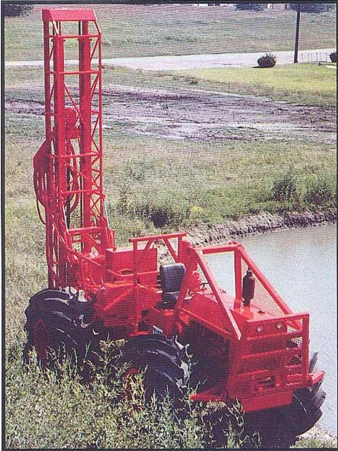
Vehicle shown with Rolligon Kingstar Geoseismic drill rig and Flo Grip Tires.
