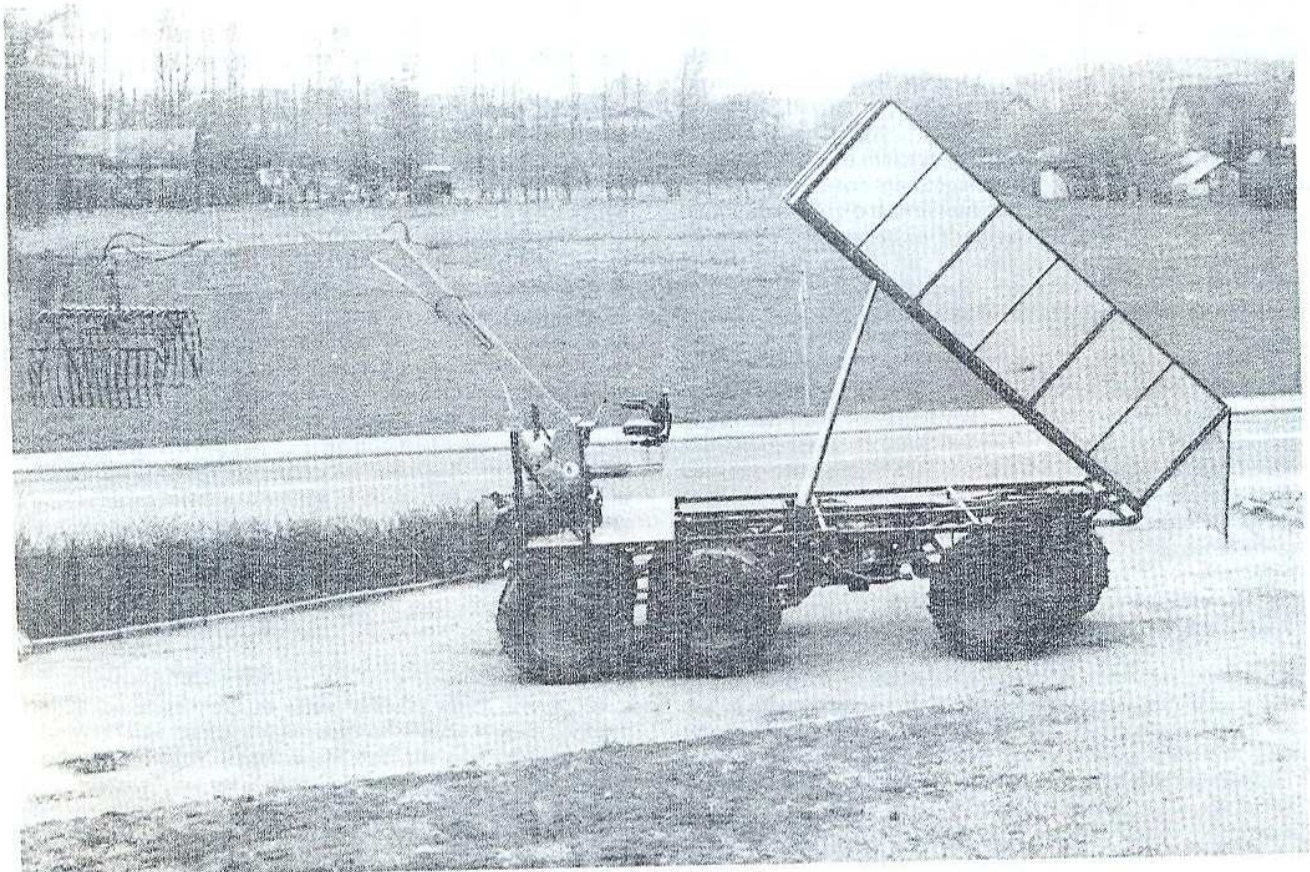
SEIGA Giant Tortoise buoyant-wheel vehicle equipped for peat bog work
