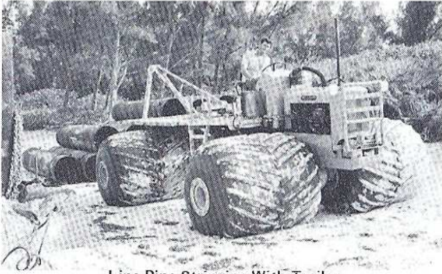
Line Pipe Stringing With Trailer
