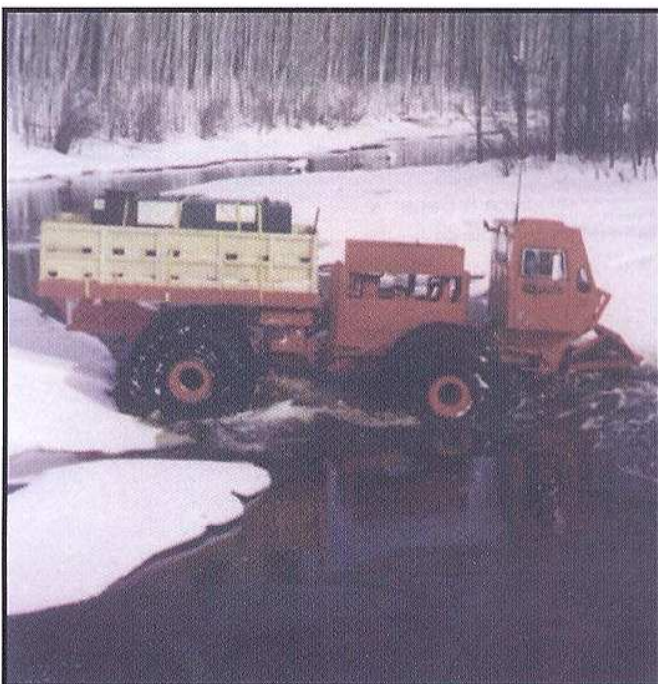
Rolligon standard 4 x 4 RA-15 vehicle with Rolligon 72 x 68 - 28 high flotation tires.
