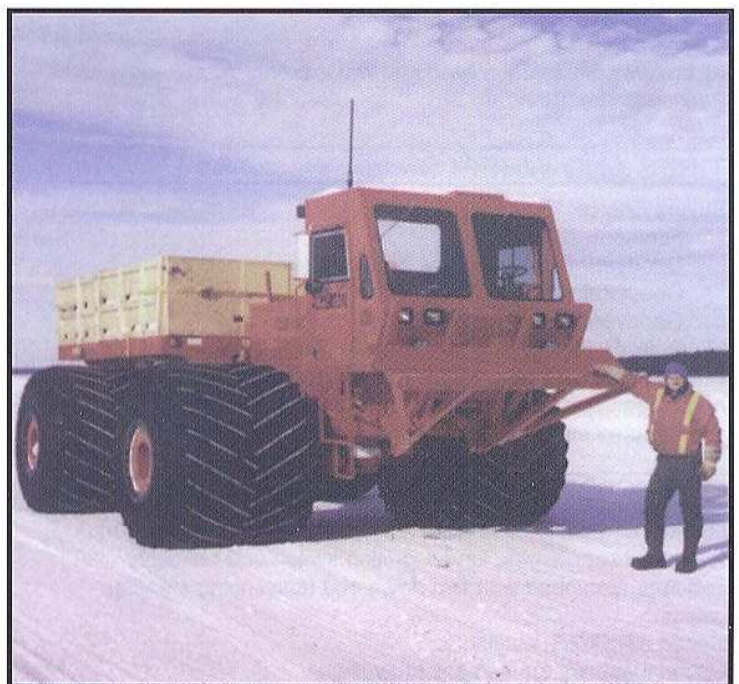
Rolligon standard 4 x 4 RA-15 vehicle with Rolligon 72 x 68 - 28 high flotation tires.
