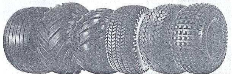
Fig. 11 - Composite photo of flotation tire tread designs (from left to right—rib, super terra grip, rawhide, xtra traction, power rib, and compass)
