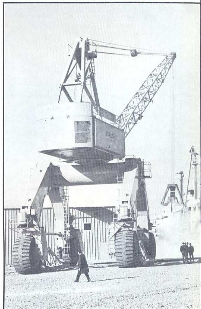
MOBILE GANTRY CRANE
