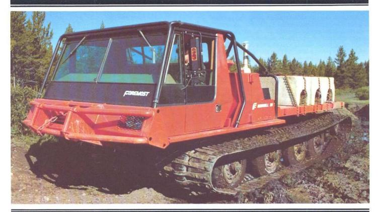
The Nodwell 110 C incorporates Foremost's latest design features including a modern all-steel four-man cab as standard, lower ground pressure, smooth underbelly, better ground clearance, reduced engine heat and noise, plus many other new features to improve performance and reduce downtime. The Nodwell 110 C is air transportable by Hercules without having to remove tracks.
