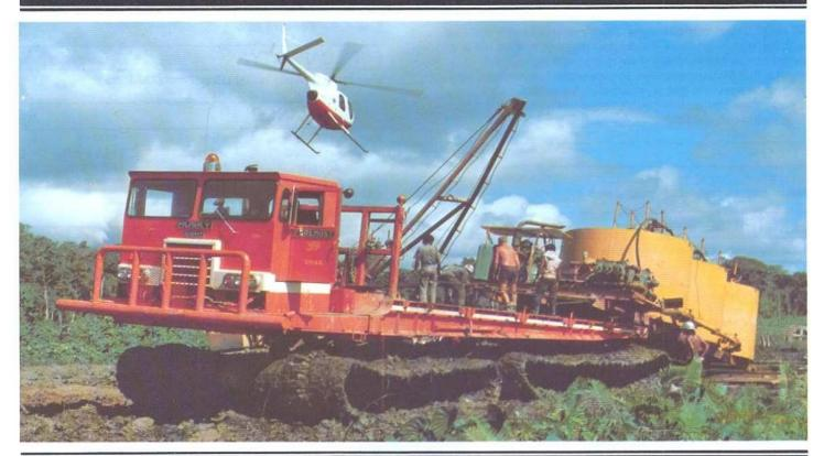
The Husky 8G is a large, four tracked vehicle designed to move heavy payloads in mud, muskeg, swamp, and snow conditions. The high deck and sealed undercarriage components provide excellent fording ability combined with high approach and departure angles. The independent crankarm suspension and flexible track provide constant ground contact, absorb shock loads and increase productivity by allowing higher travel speeds than steel tracks.
