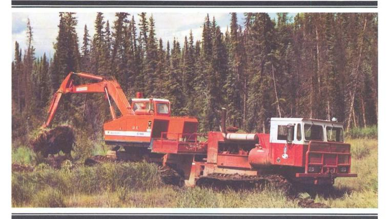
The Pioneer is a versatile, four tracked carrier, with articulated steering: with its wide tracks, the Pioneer can be readily equipped with drills and cranes, or with a deck for general heavy hauling.
