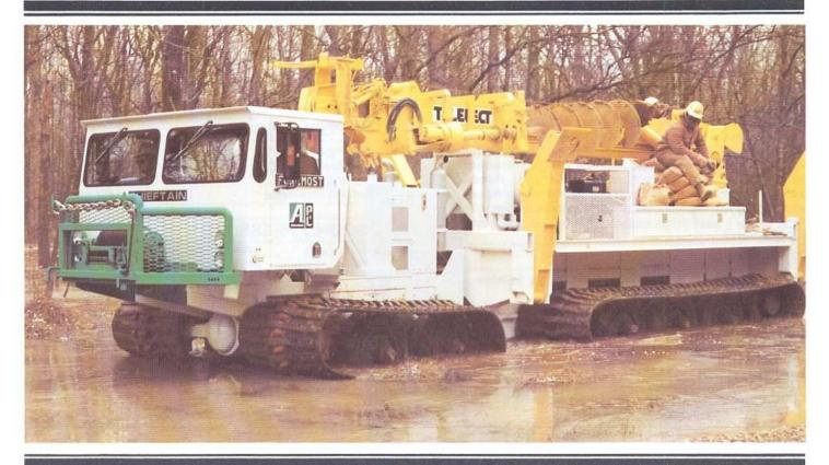
A versatile, four tracked carrier, with articulated steering, the Chieftain is ideal for mounting drills, cranes or backhoes, widely used in the petroleum, geophysical and utility industries. With the proven wide track system and high engine torque, the Chieftain provides economical transportation of cargo and personnel in marginal terrain conditions.
