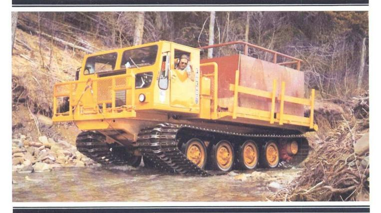
A multi-purpose two tracked vehicle, the Nodwell 110 is available in 2, 4, or 6 man cab configurations. With its low ground bearing pressure, the Nodwell 110 is ideal for use in a variety of terrain conditions. The Nodwell 110 is transportable by highway truck or Hercules aircraft.
