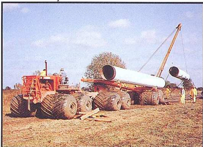
Rolligon 8x8 tractor with pipe trailer. Capacity: 20 tons.
