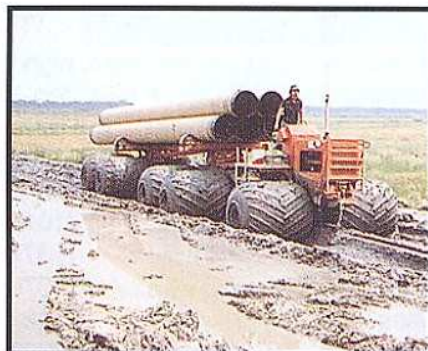
Rolligon 6x6 tractor with pipe trailer. Capacity: 15 tons.
