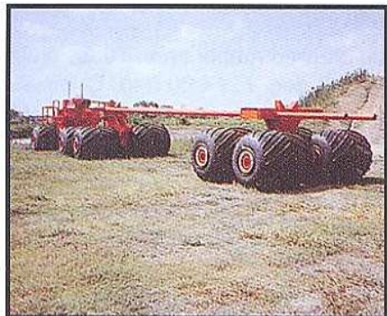
Rolligon 6x6 tractor with pipe trailer. Capacity: 15 tons.
