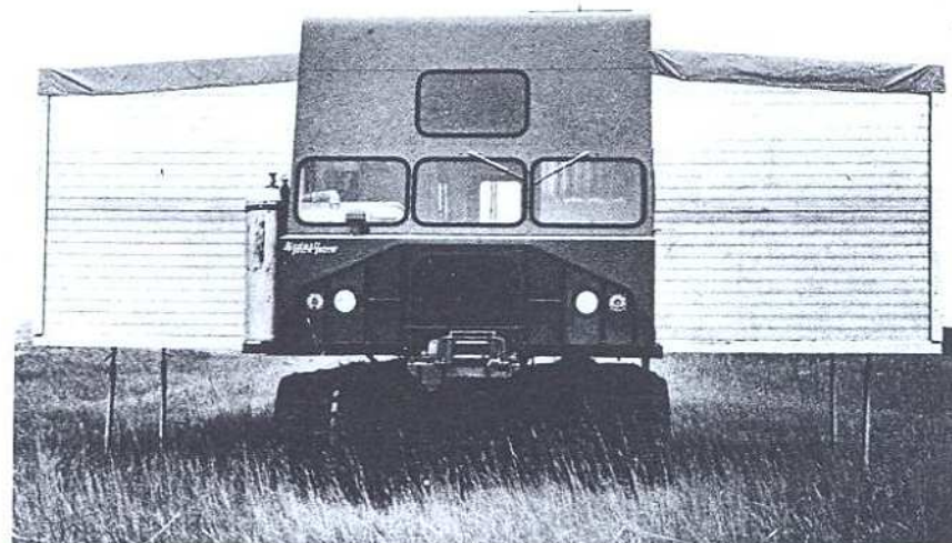
The RN 110 is pictured above with a 24 man Kitchen-Diner with expandable wall sections. For details on complete Nodwell Tracked Camp Units refer to Page 13.
