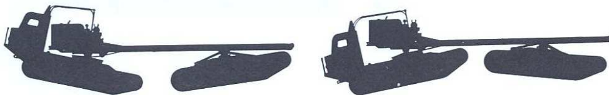
Track Units independently assume any moving angle dictated by terrain
