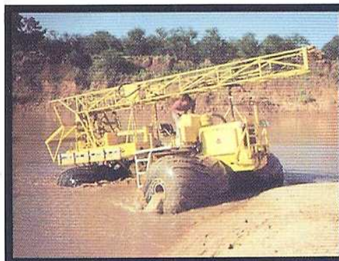
Amphibious 4 X 4 with Geophysical Drill
