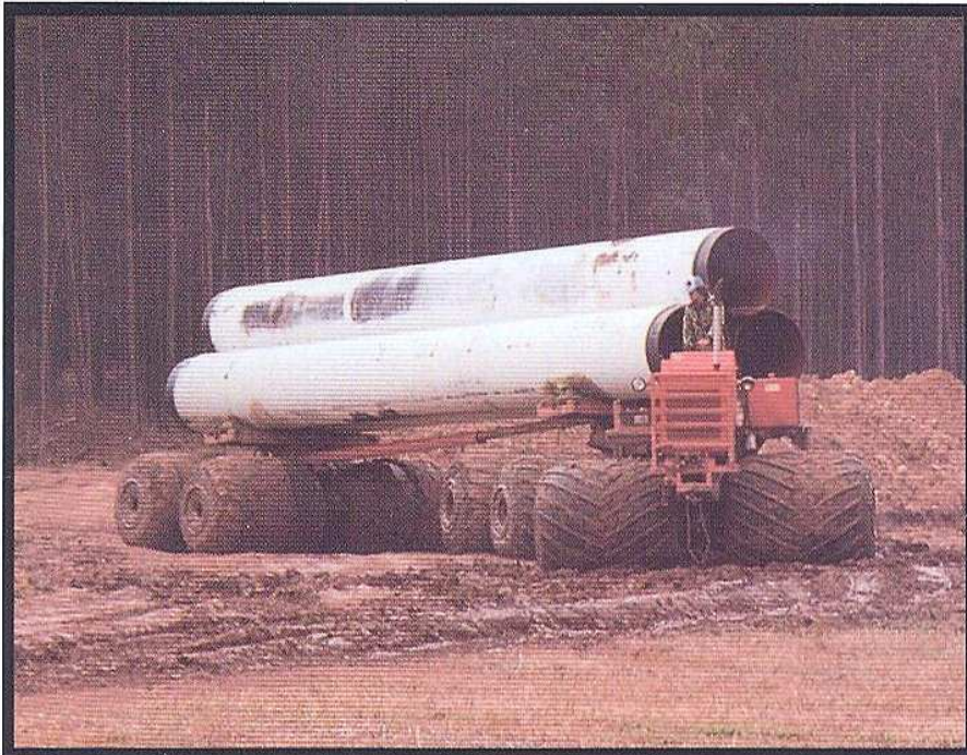
6 X 6 Tractor with Pipe Trailer for Pipeline Construction
