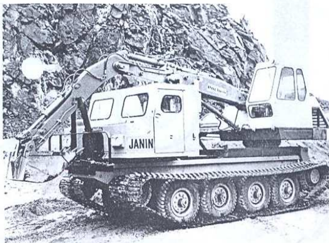
FN 240 — equipped as a steel carrier 24,000 lb. payload.
