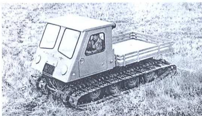
FN 15 for general survey and service duties 1500 lb. payload.
