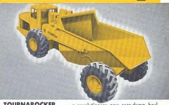
**TOURNAROCKER** . . . a revolutionary new rear-dump haul unit for use under shovel, dragline, conveyor or other loading equipment. Capacity 16 tons or 17 yards heaped. Big shovel target, 8' x 12'5" . . . 15' 11" wheelbase. Simple electric body hoist. Dumps clear over bank, tips vertical to clean fast. Turning radius 90° or 13' 9".
