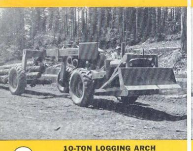
offers another profit opportunity for the 122 h.p. "D". Hoists, skids 10-ton log loads over rough terrain . . . big, low-pressure tires, and power-proportioning differential of primemover, provide easy-rolling flotation and constant-pull traction. Ample load clearance . . . 7' wide, 6'9" high inside arch. Can be used with Bulldozer on front . . . all electric control.
