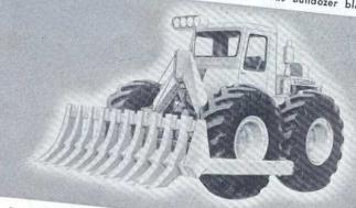
ROOT RAKE . . . offers you another low-cost, specialized tool for handling brush clearing with Tournadozer. Husky 11'8" x 3'4" rake has 10 curved teeth of 4" high-grade, heat-treated steel, placed 9" apart, for grubbing out roots, raking aside rocks. Gets the complete job done because of high-speed maneuverability and rubber tires . . . stacks brush in higher piles.
