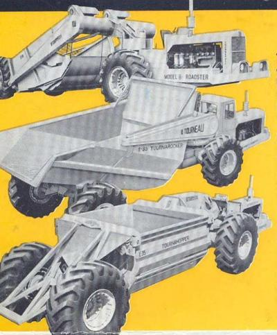
**TOURNAPULL...** electric-control scraper... 35-ton capacity... carries 30 cubic yards. Speeds to 30 m.p.h. For large volume dirtmoving, this is the answer to lowest net cost per yard. Giant tires (27.00 x 33) go anywhere. Carries more than double the load of the famous "C".
