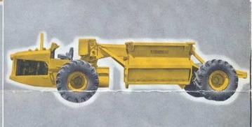
TOURNAHOPPER . . . bottom-dump hauler . . . 15-yards heaped, 16-ton capacity. Tournamatic differential, giant tires, and high clearance take it through muck and gumbo. Easy loading . . . top opening 8' x 8'. Easy to drive over windrows, clamshell-type dump-doors lift clear, give 22" clearance open. Turn radius 14'. 51% of loaded weight on drive tires.
