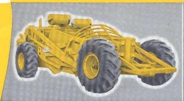
TOURNAPULL... C Roadster loads 13.5 cubic yards (capacity 16 tons). In any kind of scraper dirt on either long or short hauls, will beat all previous LeTourneau Scrapers in this size range for both output-per-day and cost-per-yard. Optional hauled units, bought as needed, cost \$4500 to \$7400, prime mover change takes only a few hours.
