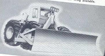
ANGLEDOZER . . . for extensive side-hill work, Tournadozer's regular Bulldozer is easily interchangeable with Angledozer blade and side arms. Husky 13' x 41½" blade can be angled 20° right or left . . . optional electric motor tilts either corner of blade on the corner of blade same A-frame and fast-acting electric PCU as Bulldozer blade.
