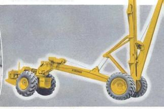
TOURNACRANE...capacity, 15 tons with full maneuverability and travel with maximum loading. Maximum lift 35', reach 35'. Sliding boom on tilting track gives unique load maneuverability for structural repair and erection. Individual electric motors control each function independently. Reaches into "impossible" places...goes anywhere through sand, mud or gumbo.
