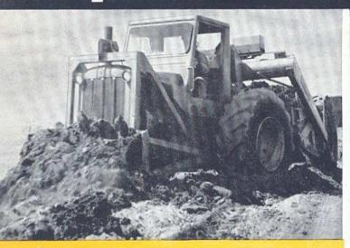
BULLDOZER on rubber-tired "D" gives you a 28 m.p.h., "drive anywhere" dozing unit for light clearing, backfilling, pusher-loading other "D's" in fleet operation. Husky 6'8 3/4 " x 2'8 1/2" blade has reversible cutting edge, replaceable tips . . . 3' blade lift . . . electric controlled. Operates independently of Carryall on rear. Bulldozer-Carryall combination often saves cost of an extra man and machine.
