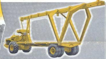
TOURNAHAULER . . . 20-ton flat-bed can take heavy mining equipment and supplies on or off highways or cross country. Traveling overhead monorail car with 5, 10 or 15-ton electric hoist optional — one-man operated from the ground by remote control or from the cab. One hauling job frequently pays for the entire-cost of the Tournahauler.
