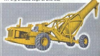
TOURNAMIXER . . . transit-mix unit of 6 or 7 yards capacity ready to go anywhere on or off highway. Mixing speed 7 to 10 r.p.m. Two discharge speeds — 7 to 20 r.p.m. No need for chutes or elevators, Tournamixer dumps directly into forms at horizontal distance of 10' 7" back of wheels or at elevations from 4' 10" to 20' 8". All electric control from driver's seat.
