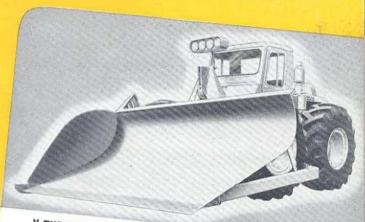
V-TYPE SNOW PLOW . . . has 12' 3" clearing width . . . flows snow 6'/2' high off ends of plowshare blade. Vertical divider plate, welded in center of "V", cuts frozen drifts . . . eliminates plowing snow back onto road when widening. Adjustable runner shoe, months! Optional electrically-operated Snow Wing available.
