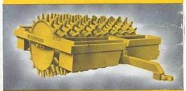
Latest type sheepsfoot roller. Accepted on U.S. Engineer Corps work, Single or multiple units . . . ground-bearing pressures up to 935# per sq. in. Standard 2-drum gives pressure from 427# empty to 935# per sq. in. loaded.
