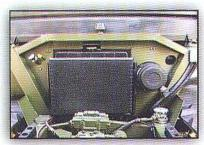
Easy daily maintenance. All routine service checks can be accessed and serviced at ground level without removing panels or tipping the cab. Convenient site gauges let you check fluid levels at a glance.
